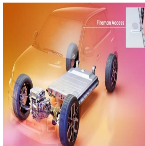
Figure 10 Chassis of an electric vehicle, which houses the motor, its batteries, and control system.
